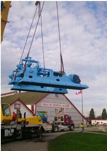
A crane lifts the 25,000 lb base of the Ice Machine onto a flatbed truck
